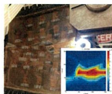
Crack detection by strain sensor array
